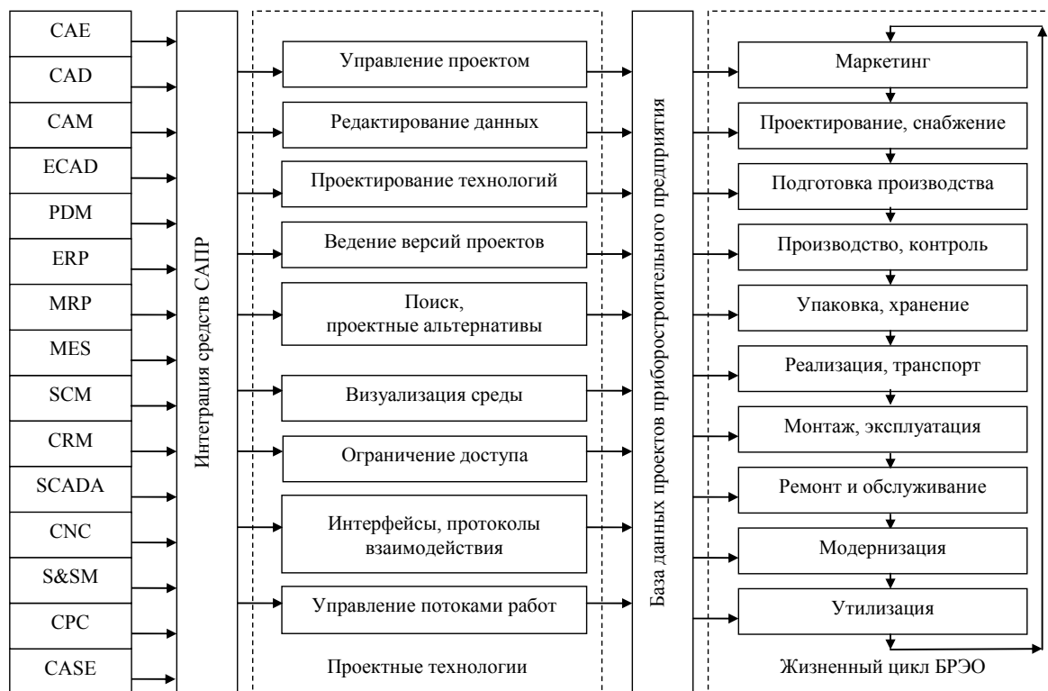
Рис. 1. Функциональная схема взаимодействия разнородных средств САПР в составе единой отраслевой САПР поддержки жизненного цикла БРЭО (CAE – Computer Aided Engineering; CAD – Computer Aided Design; CAM – Computer Aided Manufacturing; ECAD – Electronic Computer Aided Design; PDM – Product Data Management; ERP – Enterprise Resource Planning; MRP – Manufacturing Requirement Planning; MES – Manufacturing Execution System; SCM – Supply Chain Management; CRM – Customer Relationship Management; SCADA – Supervisory Control and Data Acquisition; CNC – Computer Numerical Control; S&SM – Sales and Service Management; CPC – Collaborative Product Commerce; CASE – Computer Aided Software Engineering)
